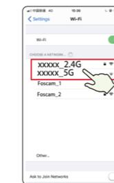
**Tips:** The camera supports dual-band 2.4GHz and 5GHz WiFi networks, so you can choose the channel with the stronger signal to use. For example, choose your SSID: XXXXX\_2.4G or XXXXX\_5G.
