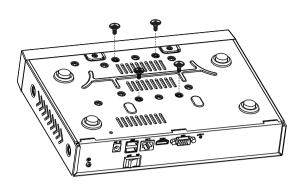
**4.** Re-install the cover of the NVR and fasten screws.
