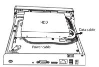
3. Place the HDD on the bottom of the device and then fasten the screws on the bottom to fix the HDD.
